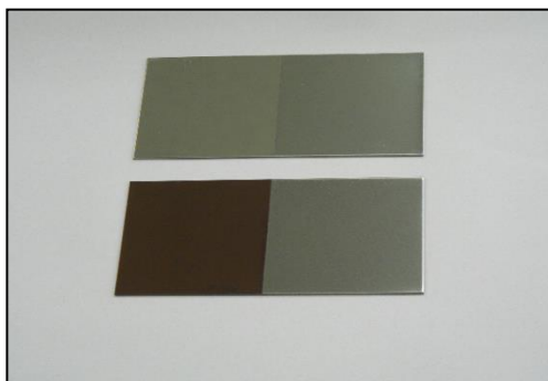
Evaluation of color changes using burner on plates with and without coatings (left: without coating right: with coating)
