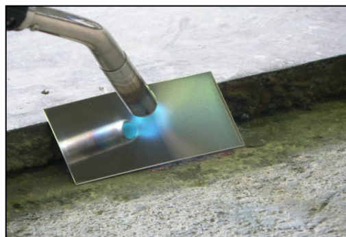
Evaluation of color changes using burner on plates with and without coatings (left: without coating right: with coating)
