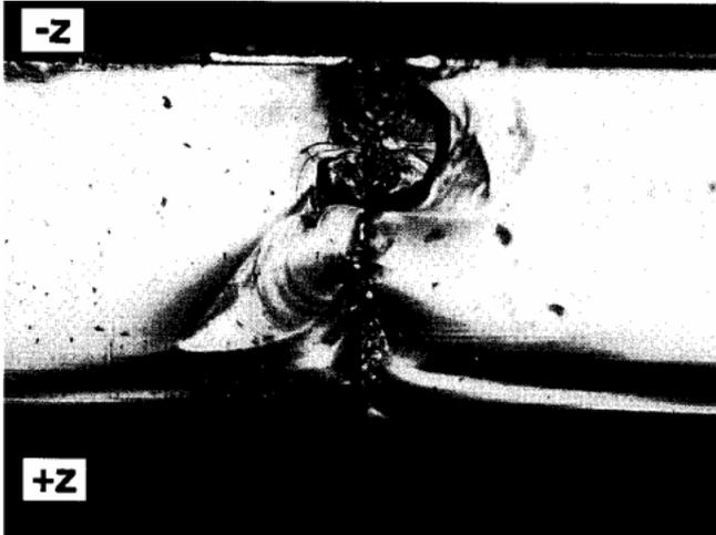
FIG. 3. Another example of a defect found on a microdomain. Thickness of the wafer is 500 μm.
