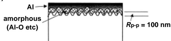
FIG. 10. Schematic depicting the process of Al film deposition on CF<sub>4</sub> plasma-etched SiO<sub>2</sub>/LiNbO<sub>3</sub>, causing Al film deterioration.
