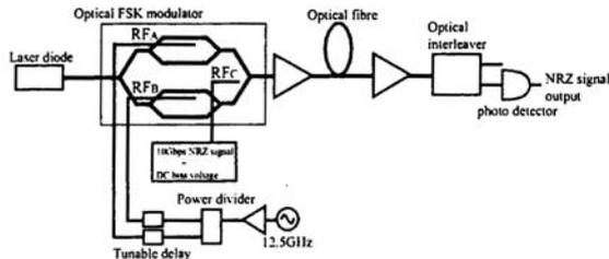
Fig. 2 Setup for optical FSK transmission
