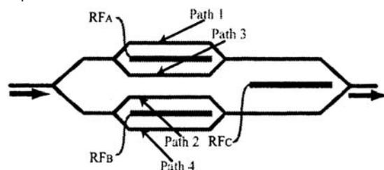
Fig. 1 Schematic structure of optical FSK modulator
