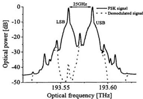
Fig. 3 Optical spectra of FSK signal (solid line) and demodulated OOK signal (dotted line)
