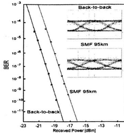
Fig. 4 BER curves and eye-diagrams
