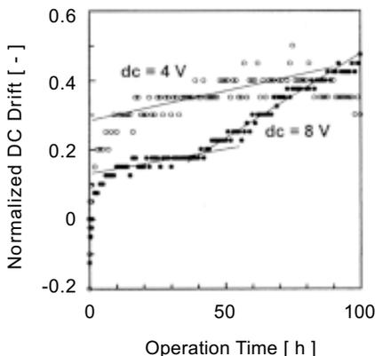
FIG. 3. Normalized dc drift measured by a fixed dc bias method at 130°C.
