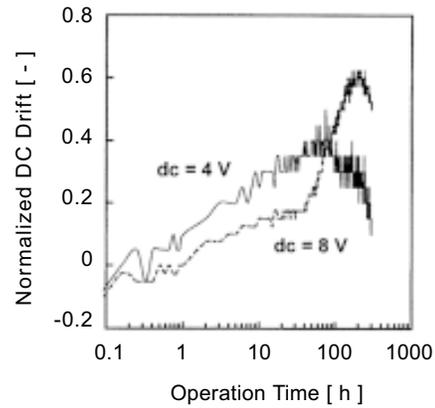
FIG. 4. Normalized dc drift measured by a fixed dc bias method at 130°C.
