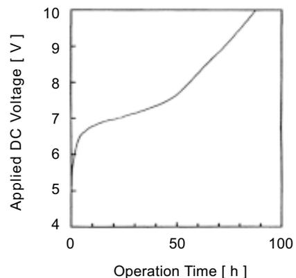
FIG. 1. Result of follow-up bias controlled operation of the modulator at 130°C with initially applied dc bias of 4.5 V.
