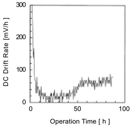
FIG. 2. Relationship between the dc drift rate and the operation time at 130°C derived from Fig. 1.
