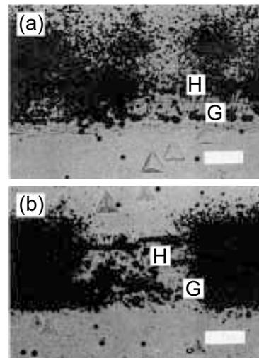
FIG. 5. Optical micrographs of the chemically etched surface of (a) the 4 V applied sample of Fig. 4 and (b) the 8 V applied sample. "H" and "G" denote the waveguide placed under the hot and ground electrodes, respectively. Bars=50 μm.
