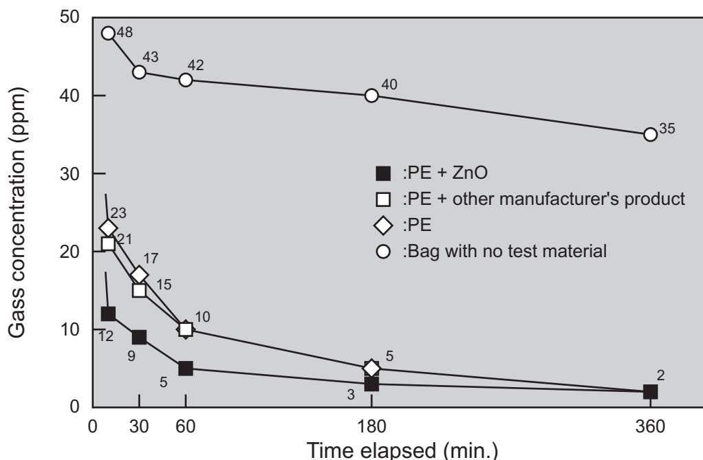
**Fig.3 Deodorant property test of films incorporated with ZnO super fine powder**
