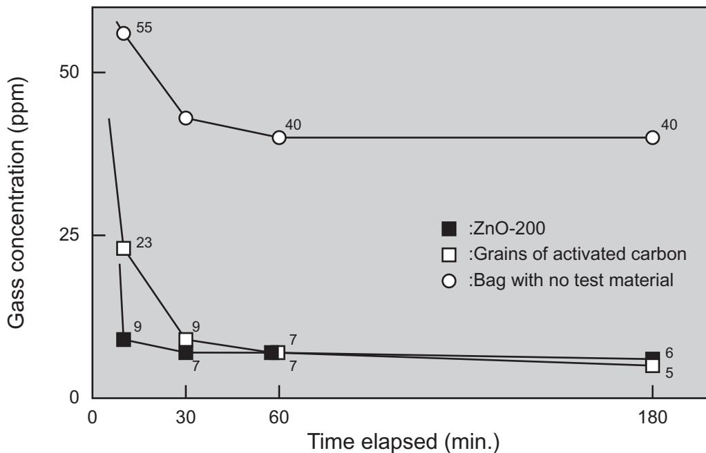
Fig.1 Deodorant property test of ZnO super fine powder with isovalerate
