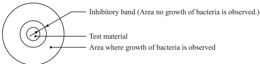
**Table 1. Antibacterial property test of zinc oxide super fine powder (halo test)**
