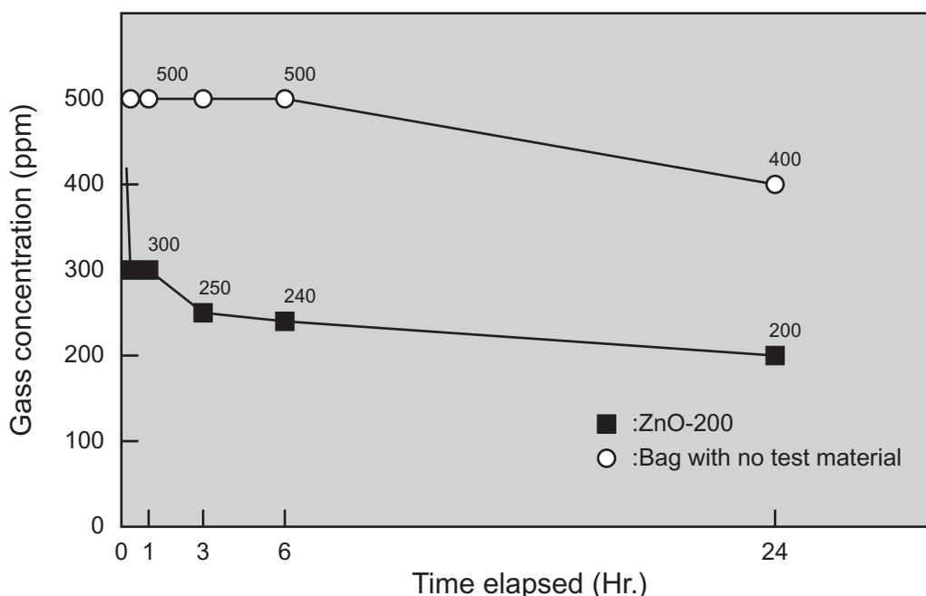
Fig.2 Deodorant property test of ZnO super fine powder with ammonia
