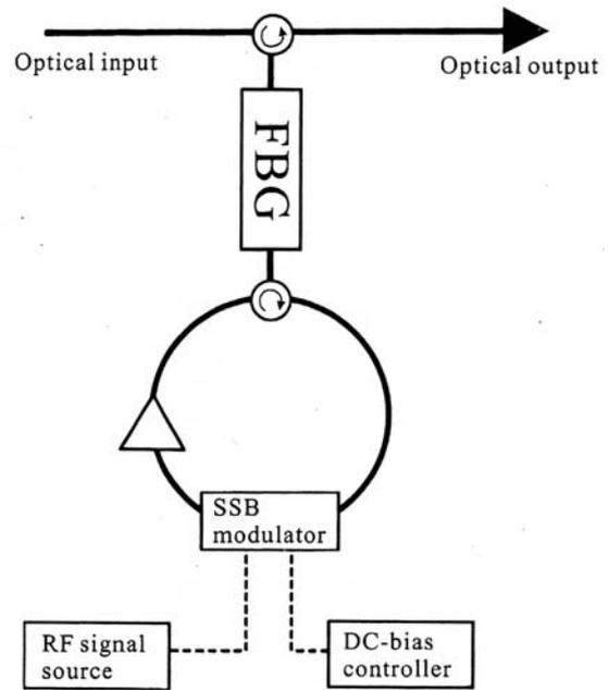
Fig. 1. Setup for our proposed delay line.
