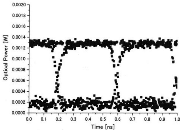
Fig. 5. Eye diagram of an input lightwave.
