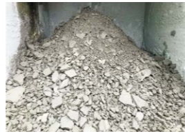
The Group’s ready-mixed concrete sludge used as raw material for recycled roadbed material
