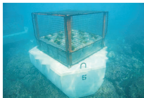
The K-hat Reef Beta, a concrete block with seaweed planted on it and covered with a net right after installation in water
