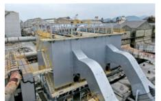
Converting Ako Plant electric dust collectors to bag filters
